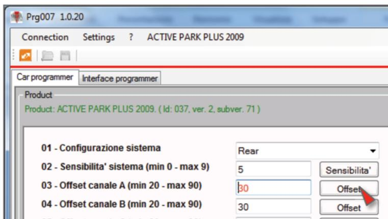
When the values have been set and recorded, press the READ key to check correct module programming.
