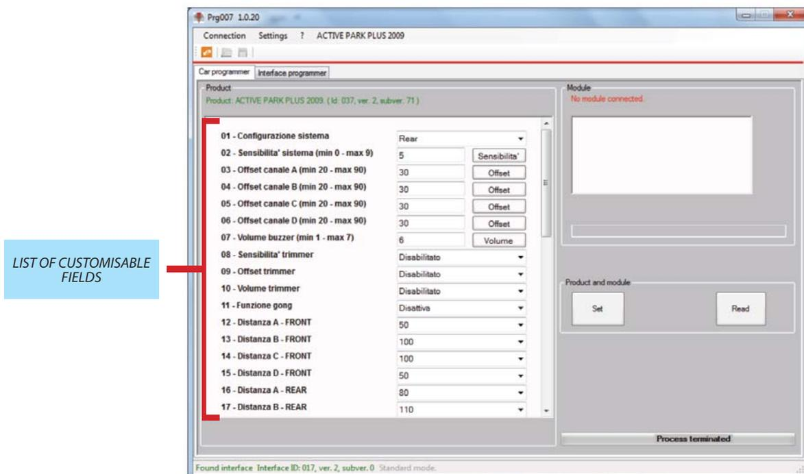
When you have made your selection from the drop-down menu, transfer the settings by using the **"SET"** command. Wait for the advancement bar to finish downloading. At this point the control unit can be disconnected and installed in the vehicle.
