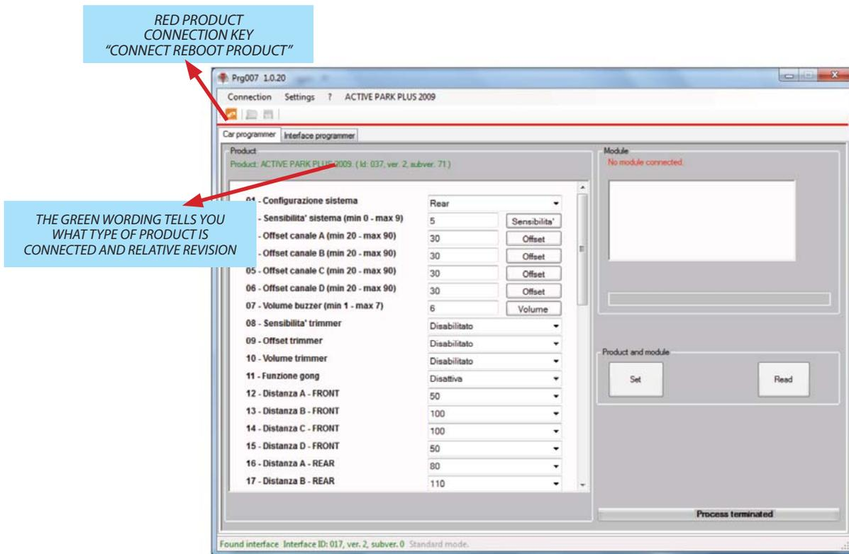
When the functions have been changed and the required module commands have been set, it is possible to transfer programming by pressing the **"SET"** command. All modified functions turn red. The **"READ"** command is used to read the settings.
